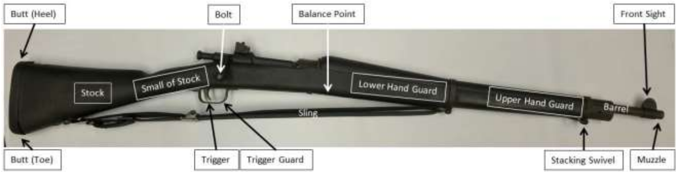
Figure 3-1b. - M1903 Springfield and Daisy Drill Rifle Nomenclature.
